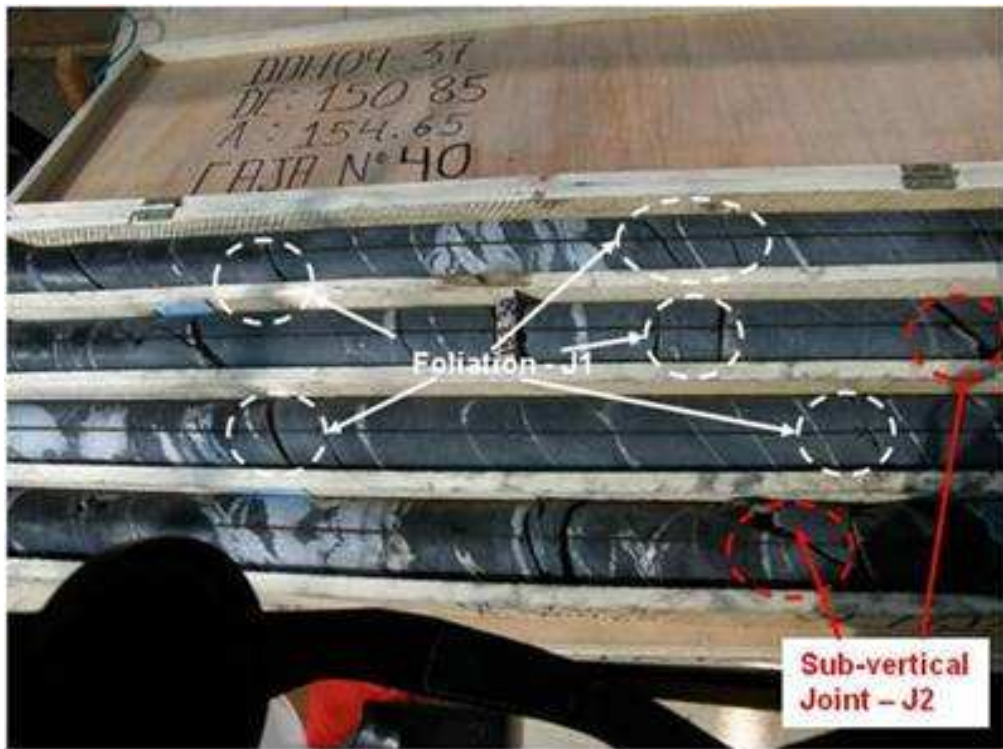
Figure 18.2.4 4 Observed Joints on the Borehole Logs
