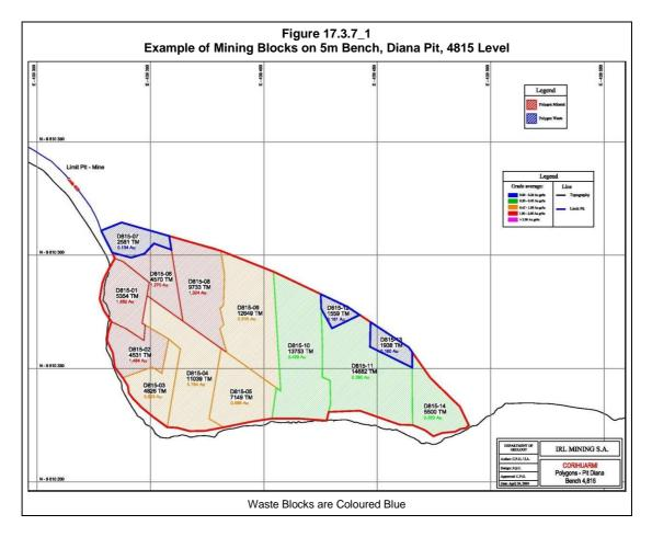
Mining is effectively restricted to the SIL which contains the economic mineralisation. The mining cutoff grades are as follows:
