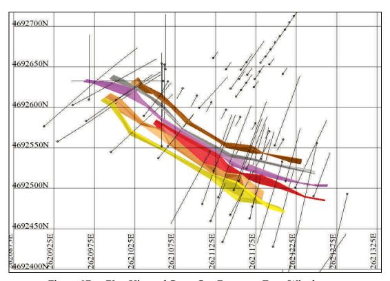
Figure 37 — Plan View of Cerro Oro Resource Zone Wireframes
