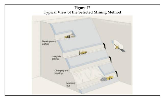
Geotechnical studies indicates that stopes that are 30m in length and 26m in height along the dip could be considered to be stable subject to the application of cable bolting to the exposures.
