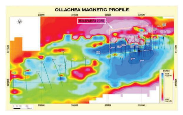
Figure 22 - Magnetic profile over a 2km strike length at Ollachea
