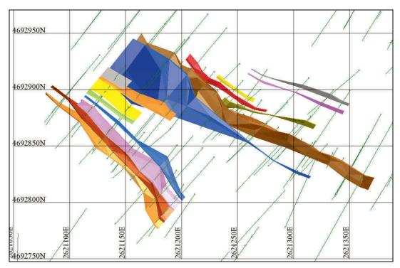
Figure 36 — Plan View of Coyote Resource Zone Wireframes
