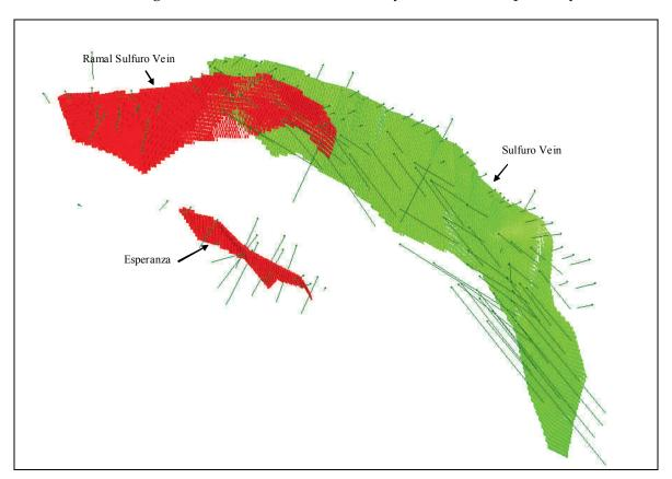
Figure 42 - Sulfuro Resource Classification (Green=Indicated, Red=Inferred) Looking NE
