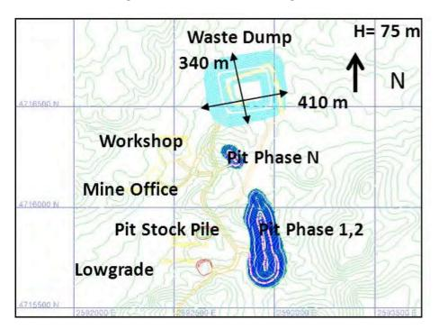
Mineable pit phases were designed based on optimized nested pit shell guidance, gold grade, strip ratio and access. Ramps in final walls have a design width of 10m and a gradient of 12%. A nominal minimum mining width of 30m was used for phase design.
