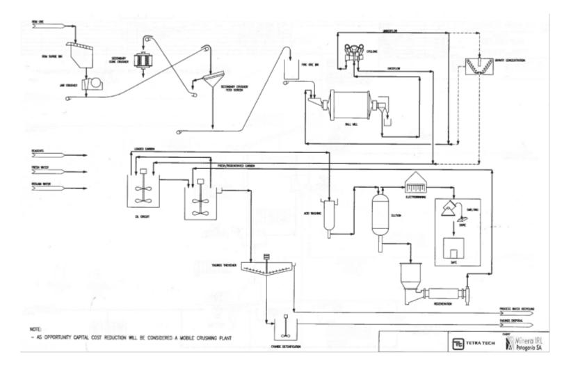
The process plant has been designed to treat gold-bearing material at the rate of 972t/d, equivalent to 350,000t/a. The major criteria used in the design are outlined in Table 44.
