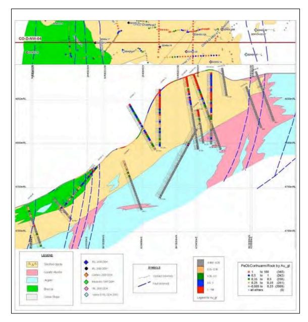
Figure 9 Corihuarmi Project - Diana Deposit - Representative Drill Section
