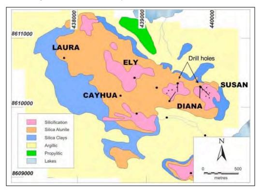
Figure 12 Corihuarmi Project - Main Block Alteration
