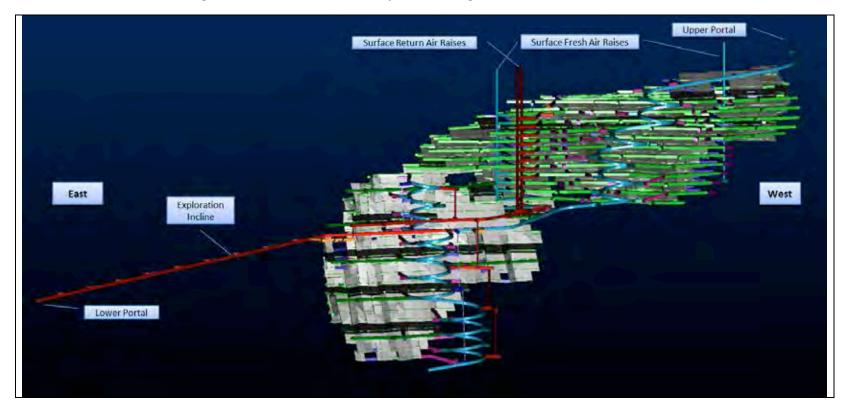
The main access to the mineralization will be via a 1.2km-long exploration access incline (1.5%) which has its portal in a valley on the north-eastern side of Cerro Joropiña and the Oscco Cachi River valley. The drive is currently being excavated and will be used for exploration drilling as well as providing the primary access and haulage drive for the planned mine. This portal (lower) will be the main mine access portal and is located above the process plant area at 2765mRL.
