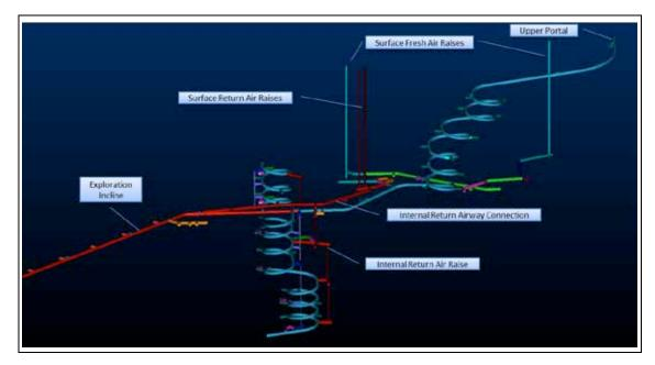
Figure 27 Primary Ventilation System
